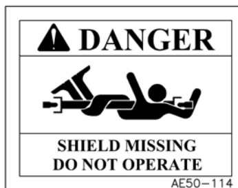
AE50-114 Danger Hazard Decal Beneath PTO Shield
