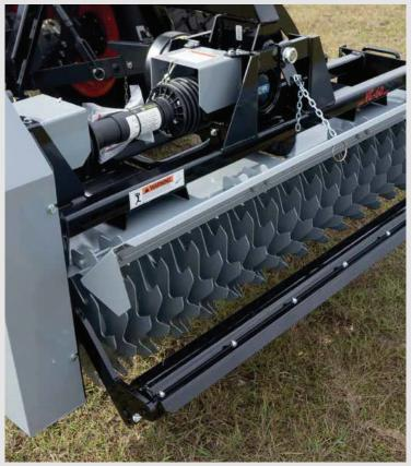
First Products introduces a smaller, compact version of the same quality. The VC40 offers tighter blade spacing from and ½"-2" spacing and an optional thinner blade, makes it the best verticutter for compact tractors.
